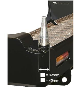
How to measure carrier pivot diameter for bearing size
